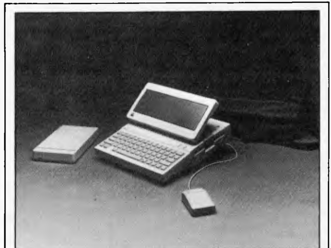
The Apple IIc personal computer with mouse, and large portable LCD display.
